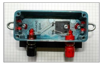
Unun connected into the antenna, ground and the feed cable:
