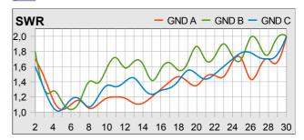
GND A (orange) GND B (green) GND C (blue) Wet ground, marsh, without counterpoise wire Dry ground, sandy ridge Average ground, field with clay
